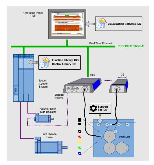
The length register adjustment normally is realized with the print cylinder drive and the side register alignement with a separate, simple actuation drive for the positioning of the print cylinder in axial direction. The position of the actuating drive can optionally be derived by the IDS and evaluated in the drive control system.
