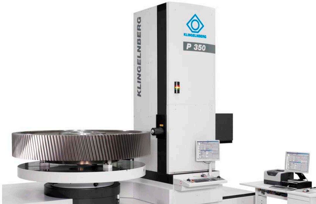
Klingelberg P350 precision measuring machine with a relatively small-sized workpiece – f. i. various gearwheels with diameters up to 3,5 m can be measured
